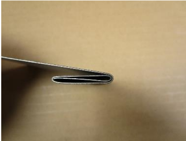
Photo No. 31 Typical T-Bend Specimen Detail
