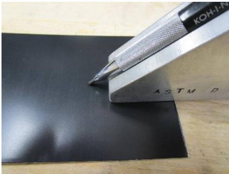
Photo No. 6 Typical Pencil Hardness Test In-Progress Detail
