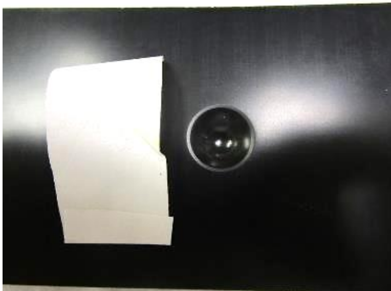
Photo No. 12 Typical Post-Tape Direct Impact Specimen Detail
