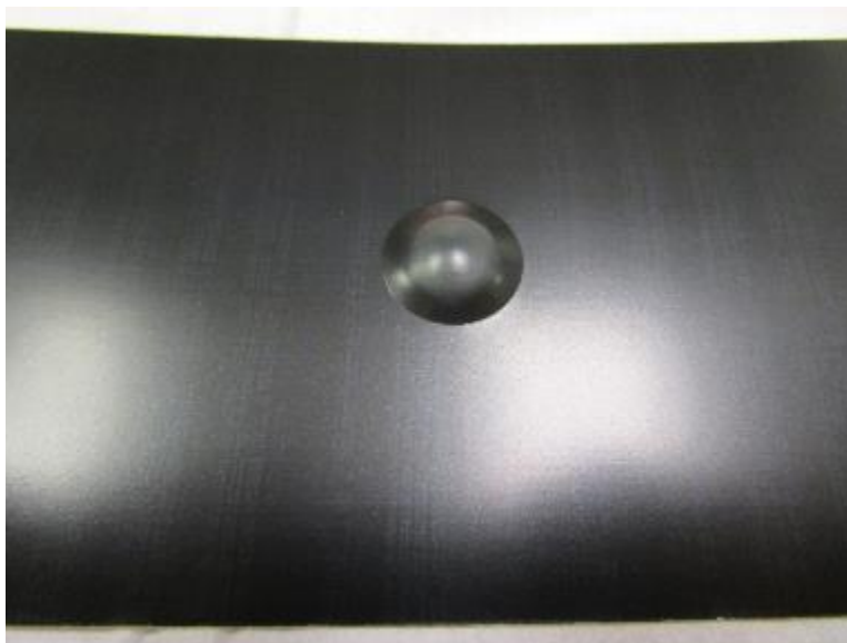
Photo No. 32 Typical Reverse Impact Specimen Detail
