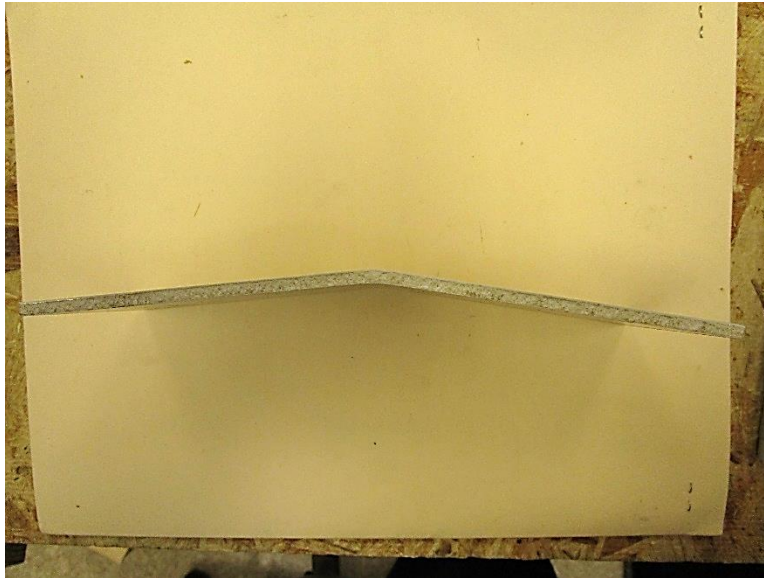
Photo No. 25 Typical Post-Flexure A2 Specimen Detail
