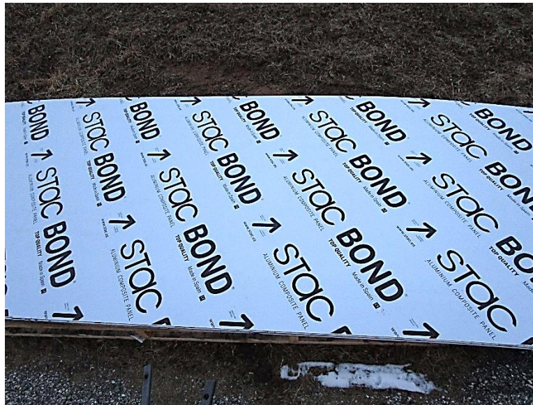
Photo No. 1 ACM Panels As-Received
