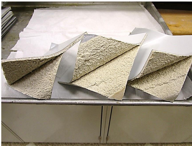
Photo No. 30 Stability A2 Specimen Failure Detail
