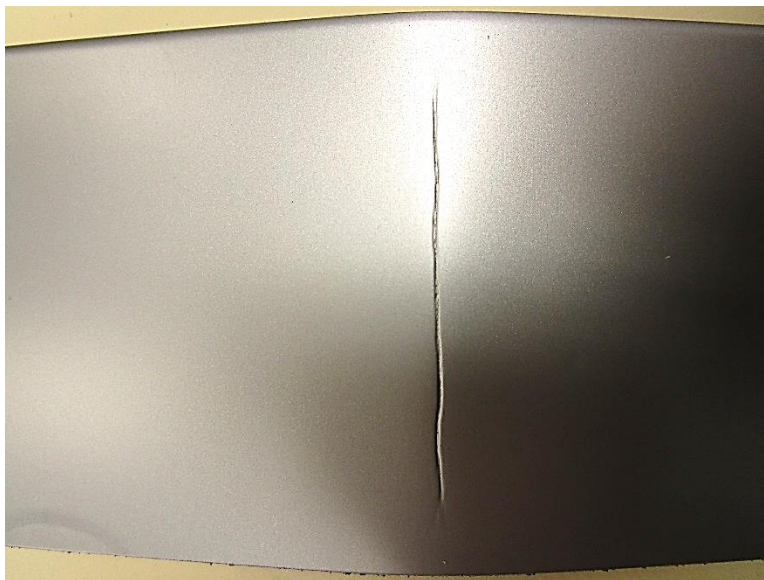
Photo No. 24 Typical Post-Flexure PE Specimen Failure Detail
