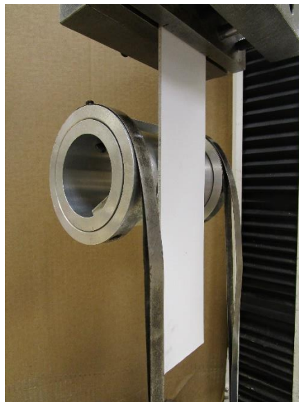
Photo No. 12 Typical Climbing Drum Peel Test In-Progress Detail
