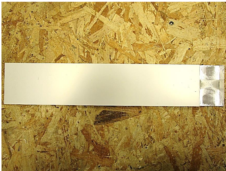
Photo No. 10 Typical Climbing Drum Peel Specimen Detail
