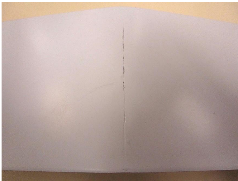
Photo No. 22 Typical Post-Flexure FR Specimen Failure Detail
