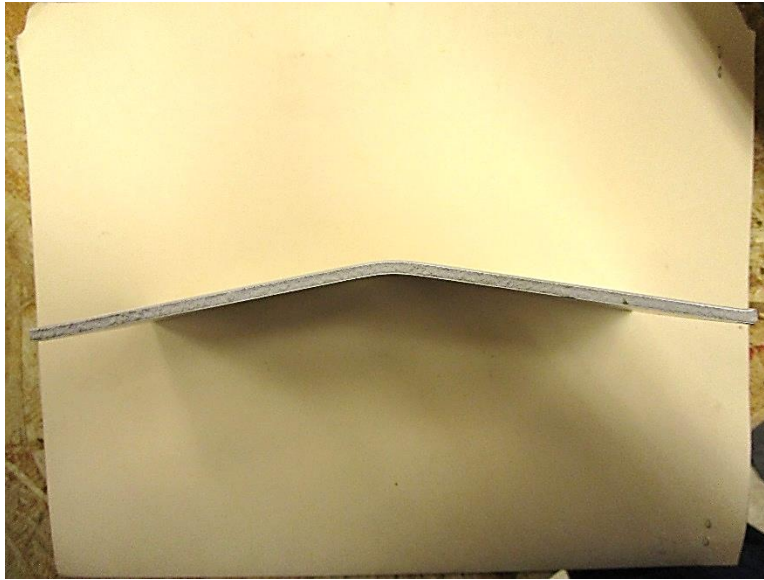
Photo No. 21 Typical Post-Flexure FR Specimen Detail
