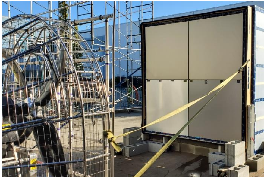
Test Setup – Dynamic Water - AAMA 501.1
