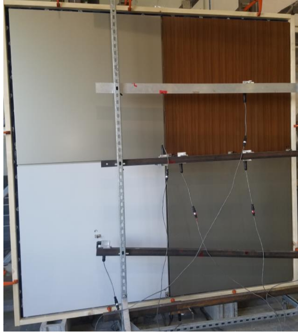
Test Setup – Uniform Load - E330
